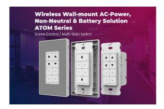
MAGTECH introduces the ATOM - a wireless wall switch, compatible with zigbee Pro or Bluetooth 5.0, with multiple scene controls and built-in relay for on and off control in 2-8 button models. It is suitable for multi-gang installation with 110-277V input. It supports low power loads and features power failure memory – returning to set level at moment of failure.
