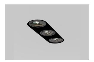
Solo from Glint is a point-source luminaire that can be optically aimed without moving the luminaire itself. An internal mechanism controls the direction of light with no tilting components. Solo has an inward-facing LED, advanced low-scatter optics and an adaptive baffle for low glare with consistent color uniformity and beam quality. The core module is only 2" wide and 5/8" deep, enabling many products variants. It is compact, glare-free and fully-adjustable.
