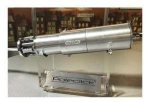
Maintenance on street and area lighting is often done at a 6-12 meter height, with 2 workers using hand tools taking 20-25 minutes. Installing a Poleclick connector enables replacement of LED luminaires within 5 minutes. It is tool-free, structurally strong, unnoticeable with the same pole diameter, universally compatible with lighting and poles brands, versatile for horizontal and vertical application and safe.
